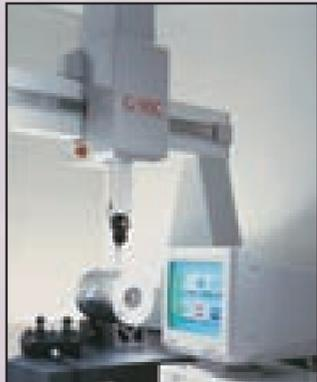
The Coordinate Measuring Machine is used for critical measurement of complex parts. This equipment provides statistical process control (SPC) capabilities, is programmable and automated, resulting in the highest level of measurement confidence.
