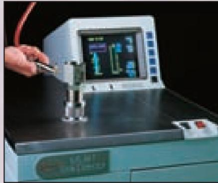
A Mass Spectrometer Leak Detector is used for non-destructive leak testing, quantitatively measuring leak rates in the range of 10 to 6 X 10<sup>-11</sup> atm. cc/sec. of air.
